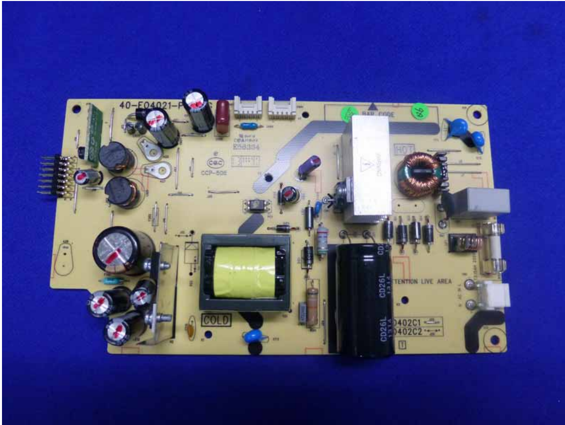
Figure 16 Frontside of the Power Board
