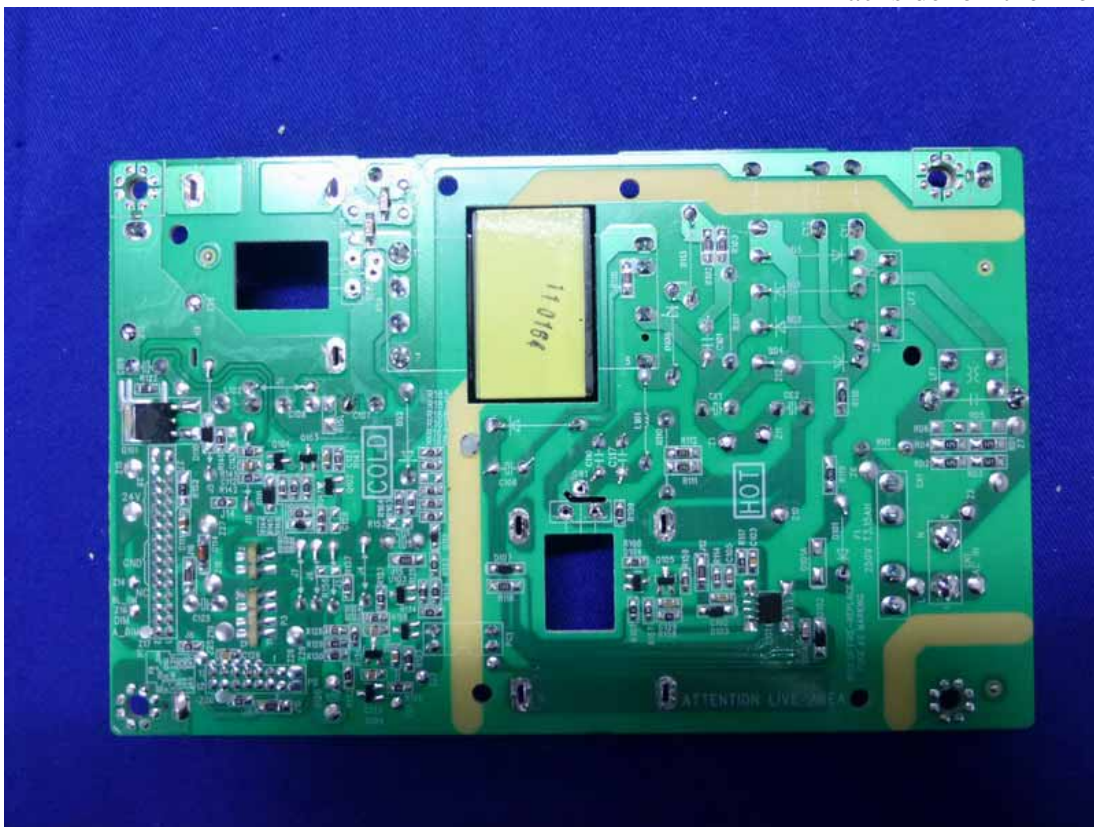
Figure 22 Backside of the Power Board
