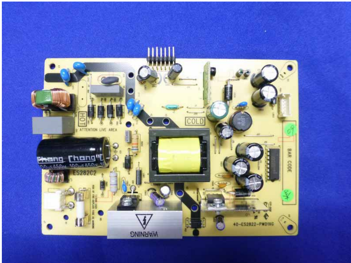
Figure 17 Frontside of the Power Board
