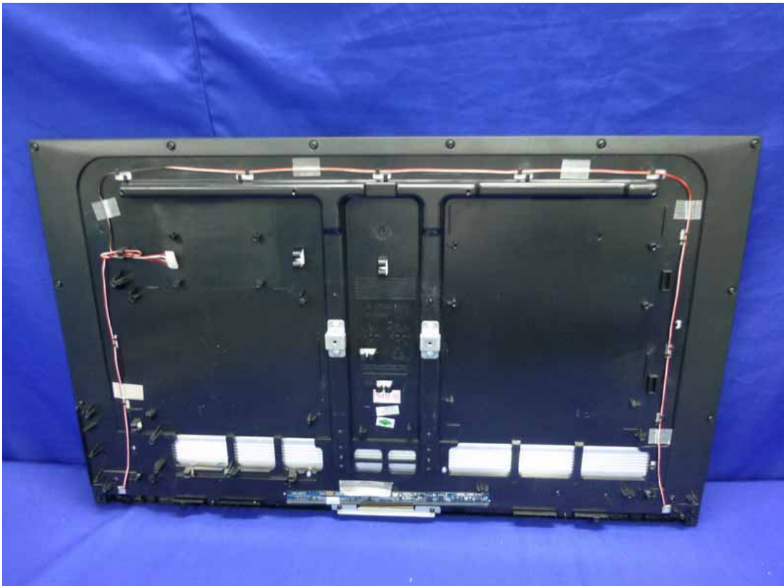
Figure 12 Backside of the LCD Panel
