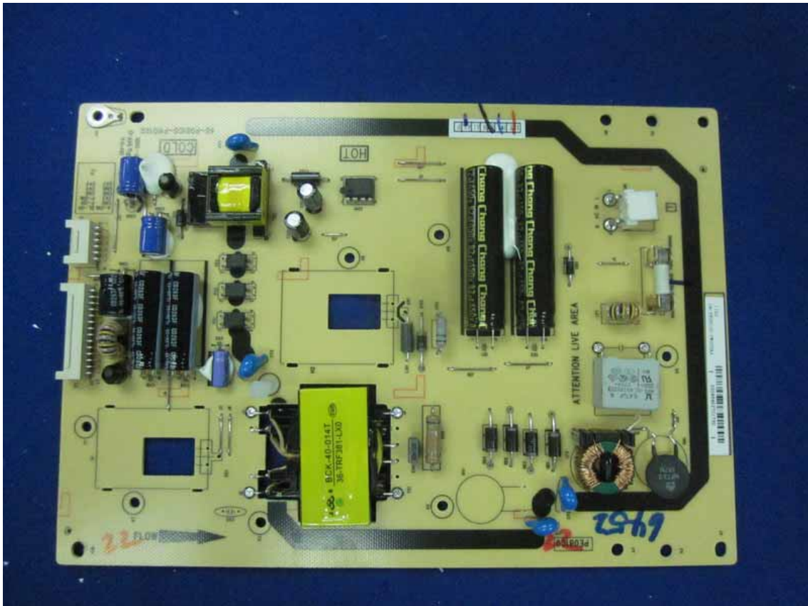
Frontside of the Power Board
