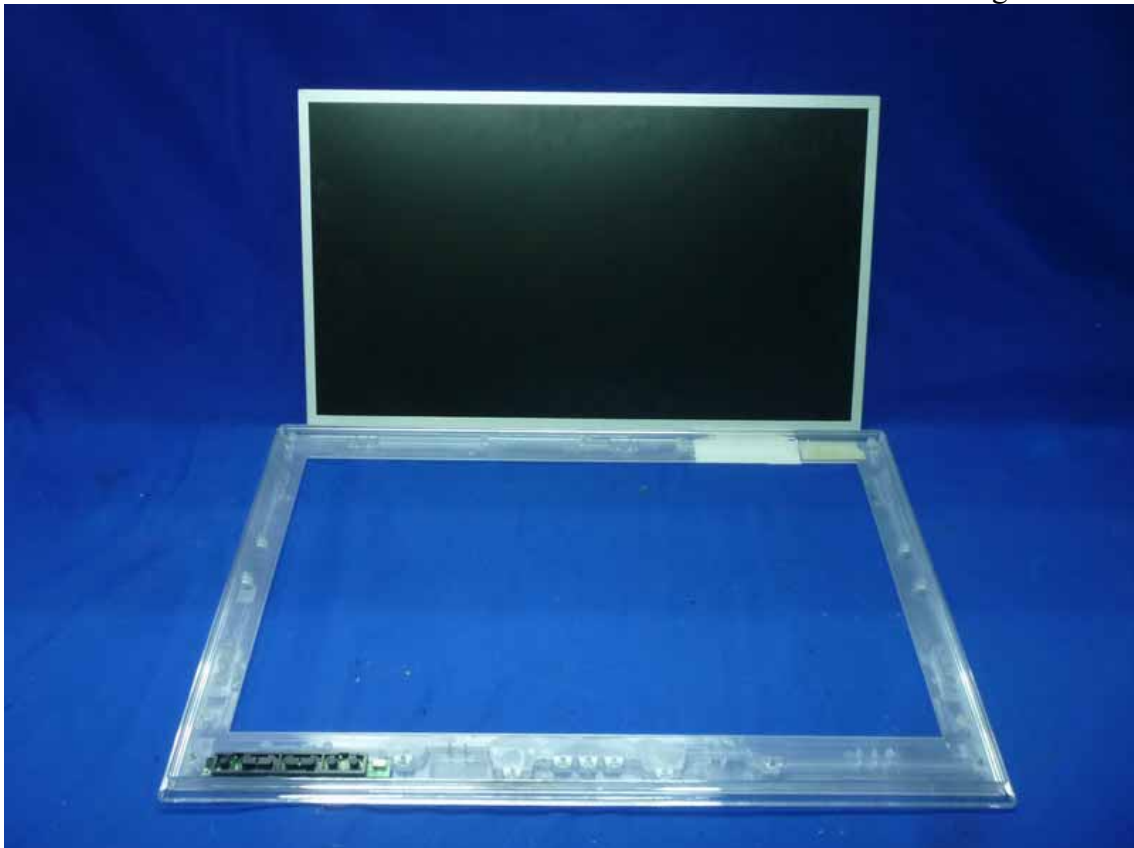
Figure 8 Inside Configuration of the EUT
