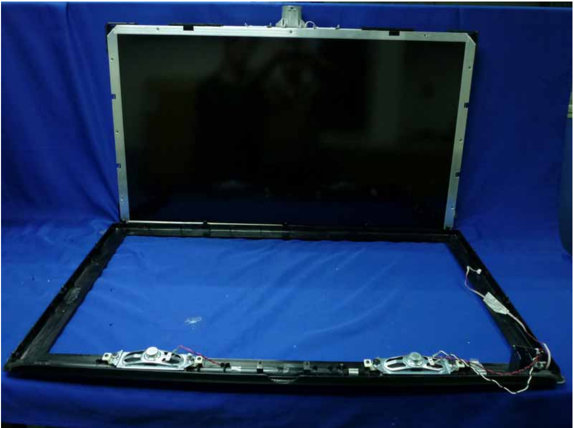
Figure 6 Inside of the EUT
