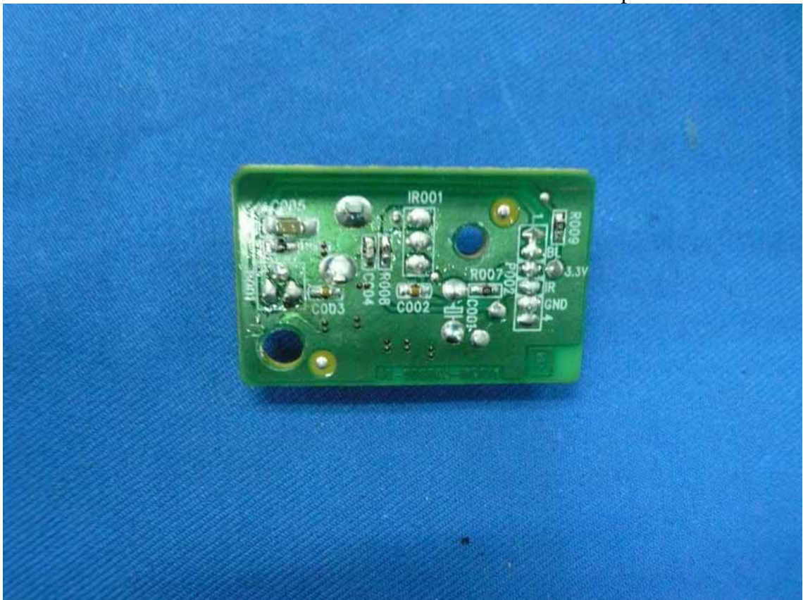
Figure 24 Component side of the PCB
