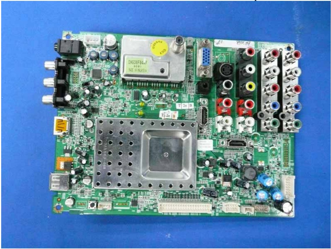
Figure 18 Component side of the PCB
