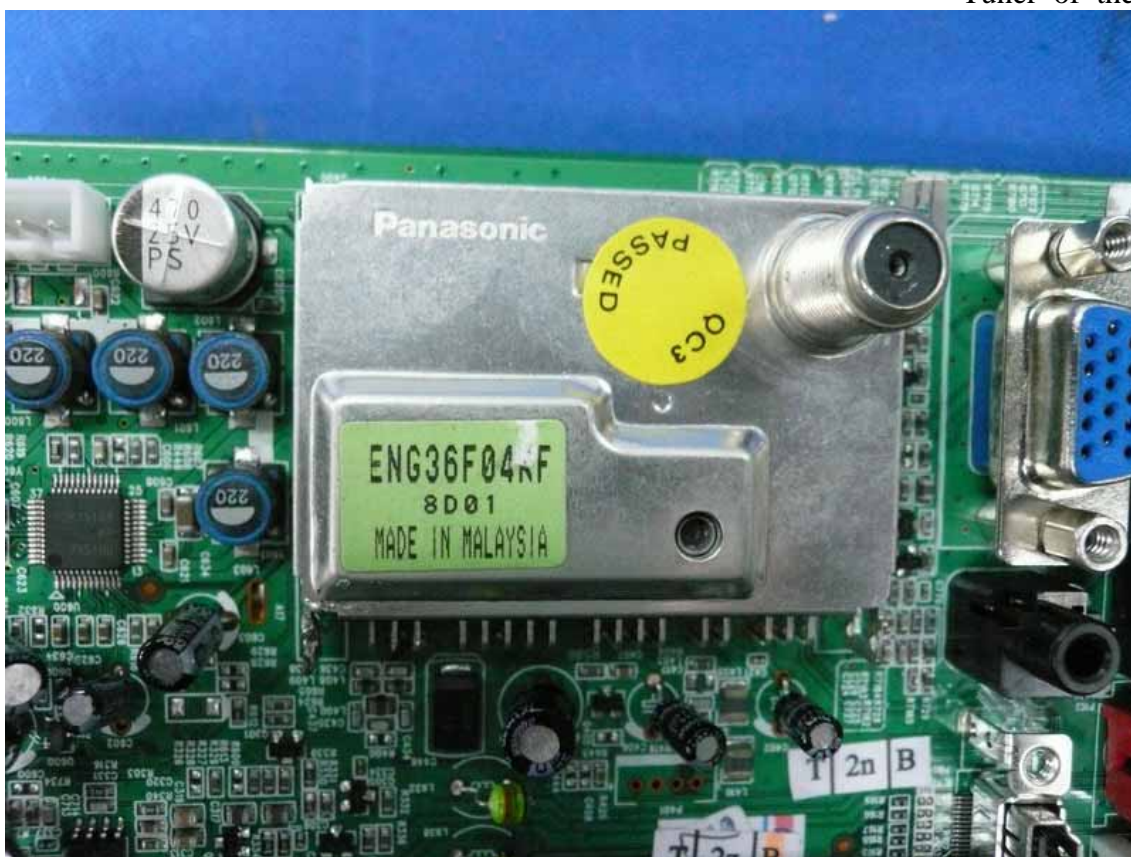
Figure 16 Tuner of the PCB
