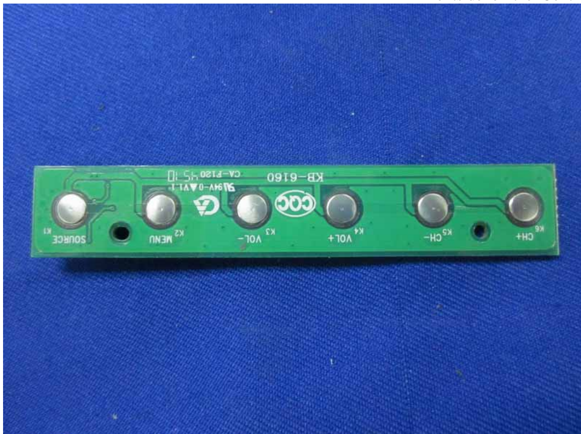
Figure 18 Frontside of the Control Board
