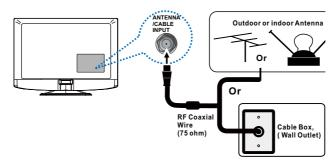
Connect the RF coaxial cable on your home outlet to the **ANTENNA**/ **CABLE INPUT** jack of this unit.
