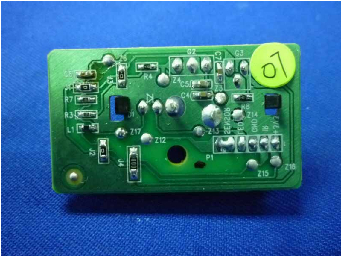
Figure 18 Backside of the Control Board
