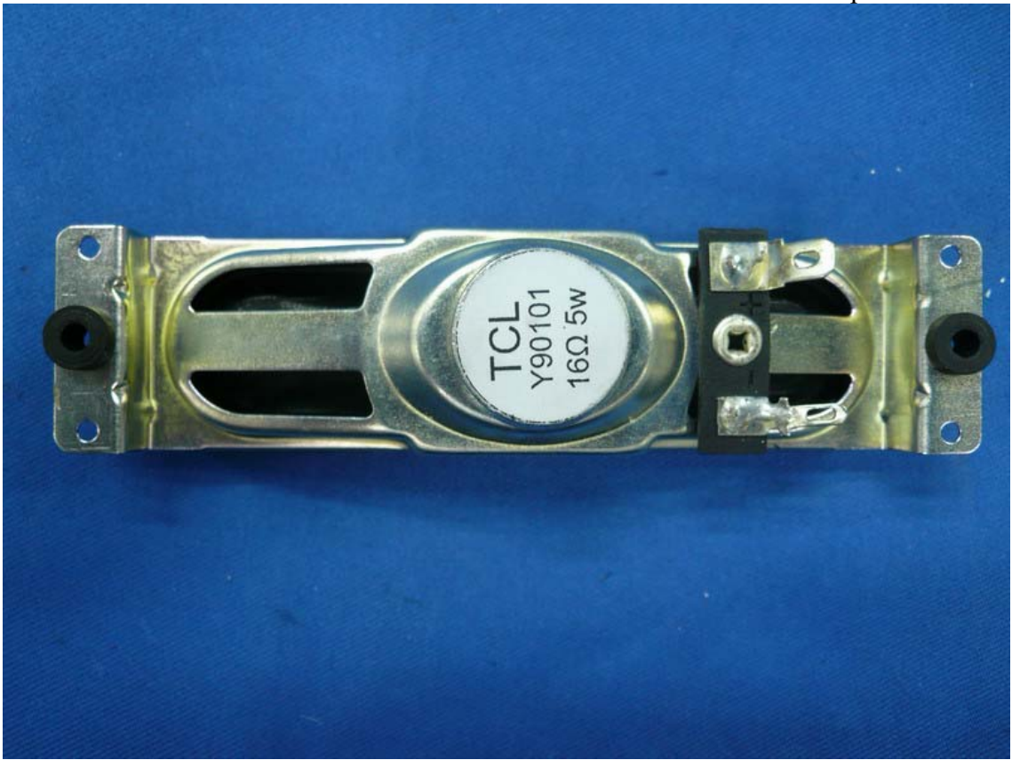
Figure 12 Speaker of the EUT
