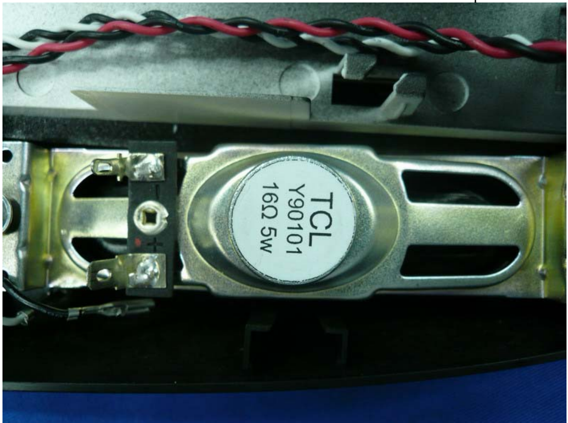
Figure 10 Speaker of the EUT
