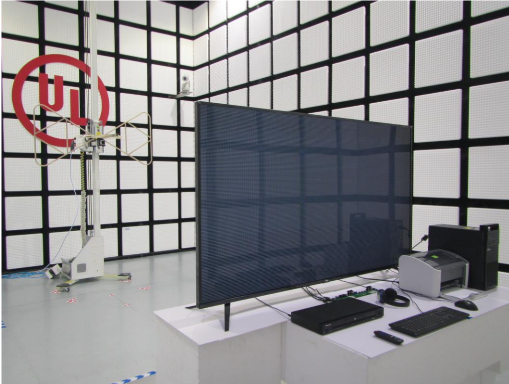
Radiated Disturbance below 1GHz – front view
