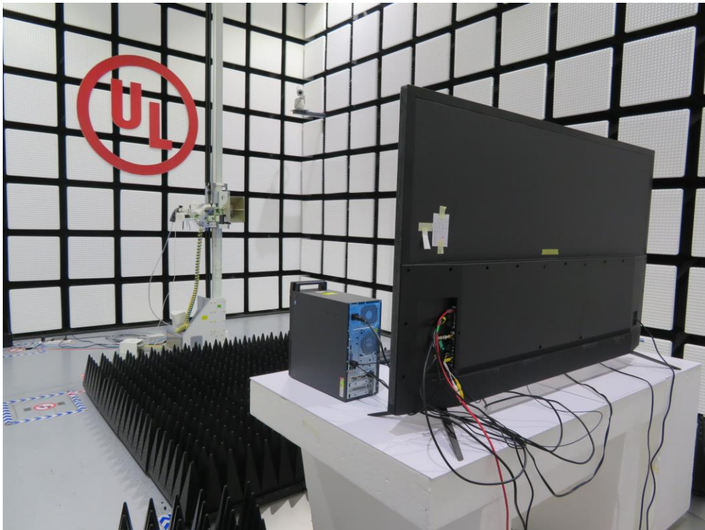
Radiated Disturbance above 1GHz – rear view
