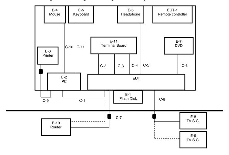
The EUT has been tested as an independent unit together with other necessary accessories or support units. The following support units or accessories were used to form a representative test configuration during the tests.
