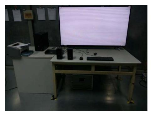
1.1. Set-up for conducted emission at the mains terminals test
