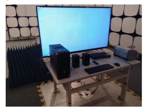
1.3. Set-up for radiated emission test (Above 1GHz)
