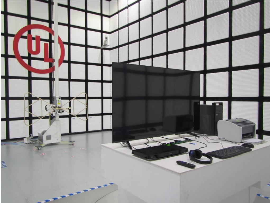
Radiated Disturbance below 1GHz – front view
