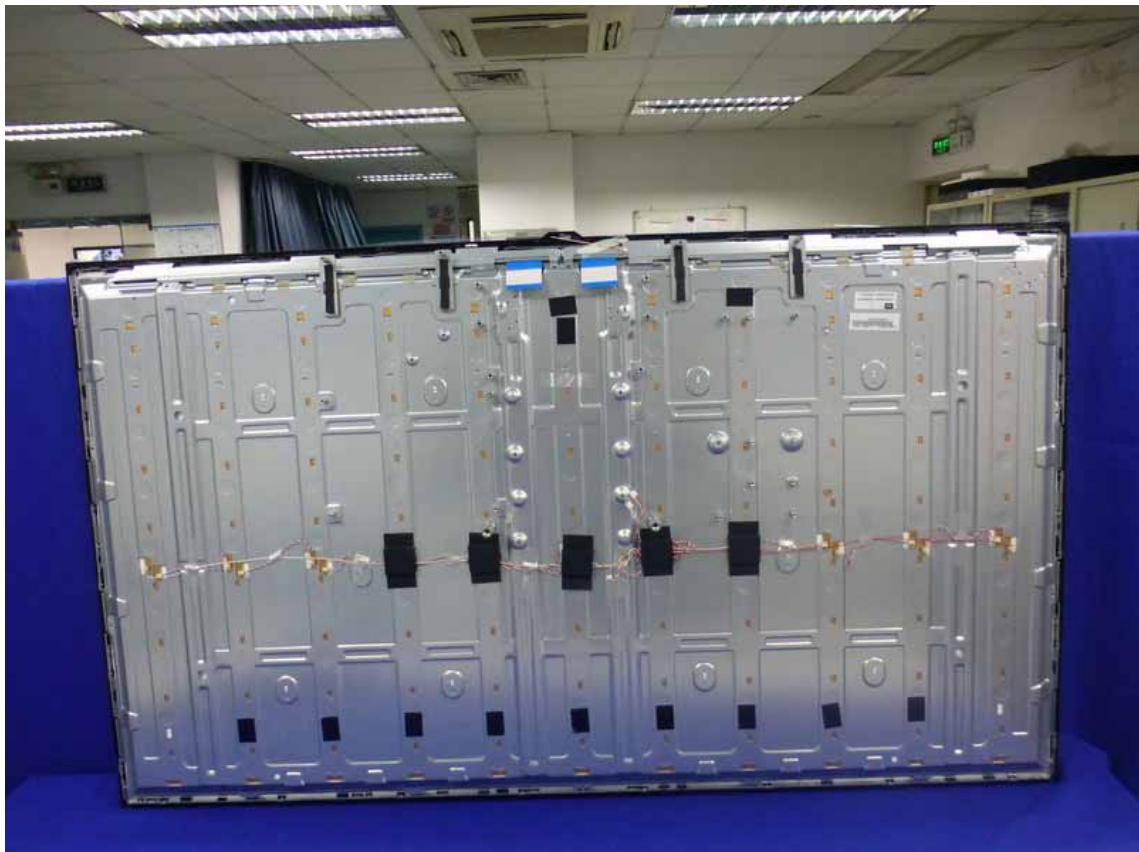
Figure 14 Backside of the LCD Panel
