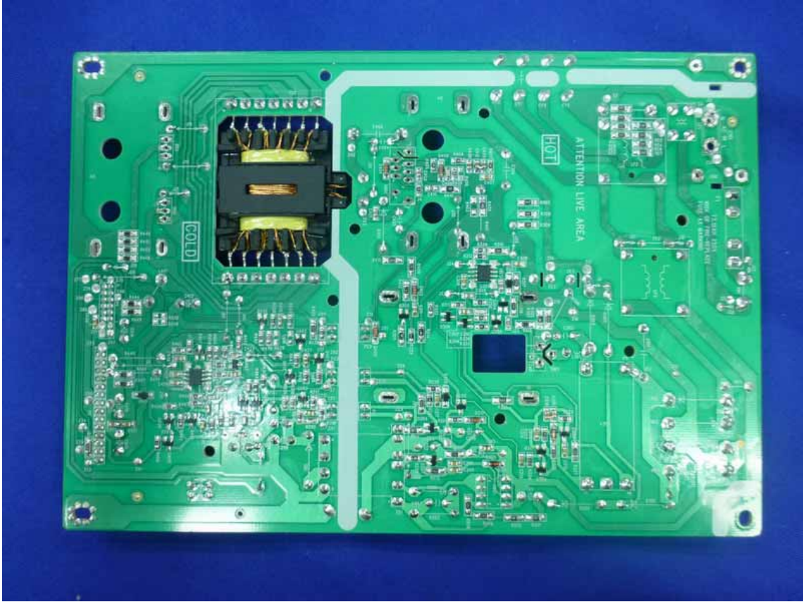
Figure 25 Frontside of the Power Board
