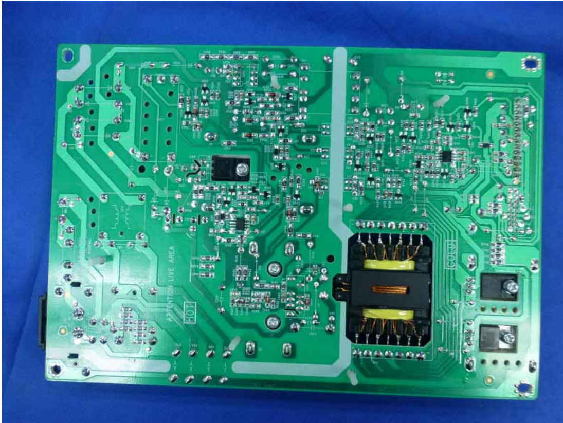
Figure 19 Backside of the Power Board
