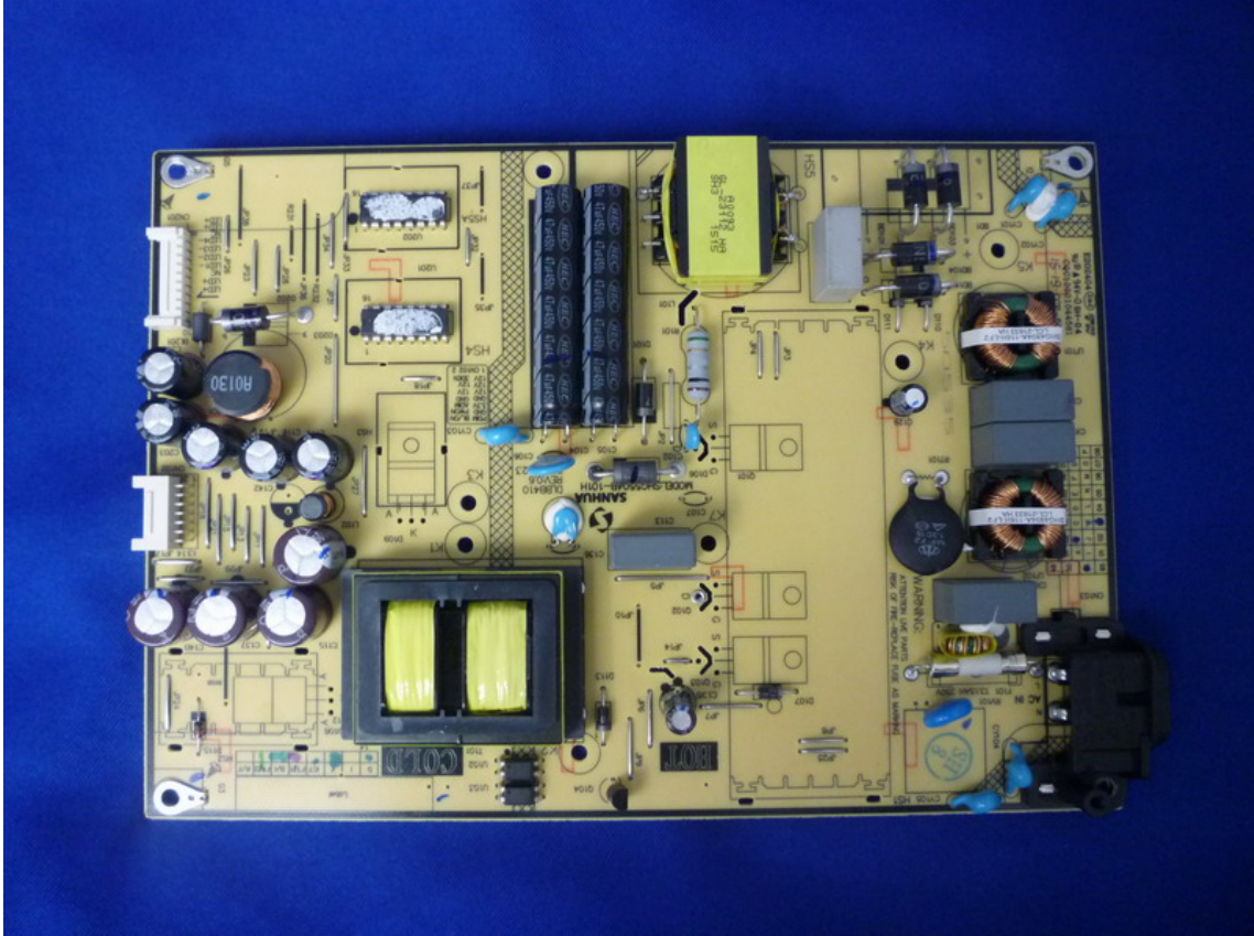
Figure 11 Frontside of the Power Board
