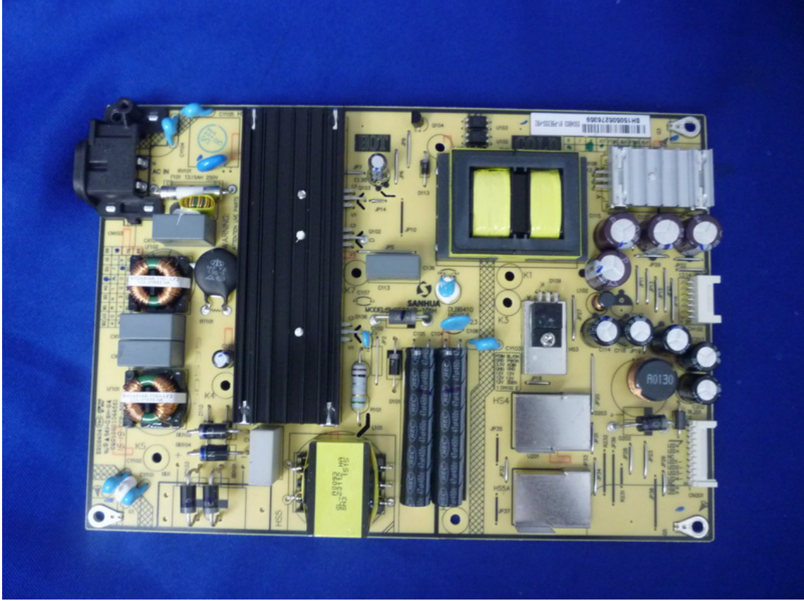
Figure 9 Frontside of the Power Board
