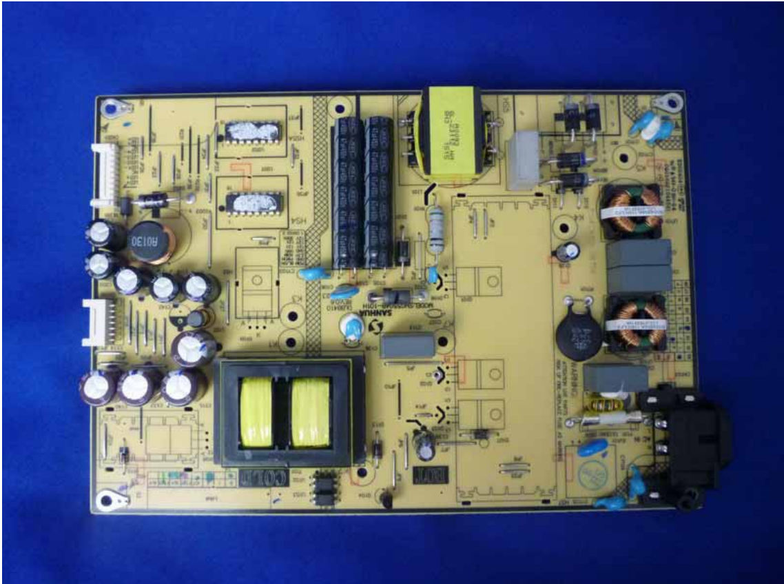
Figure 12 Frontside of the Power Board
