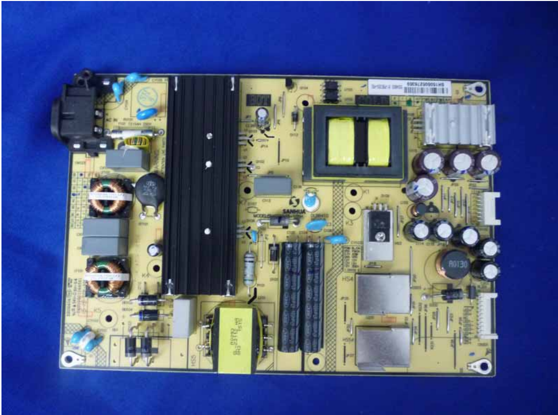
Figure 10 Frontside of the Power Board
