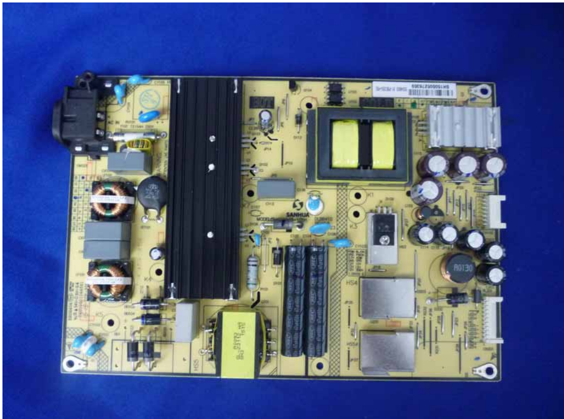
Figure 10 Frontside of the Power Board
