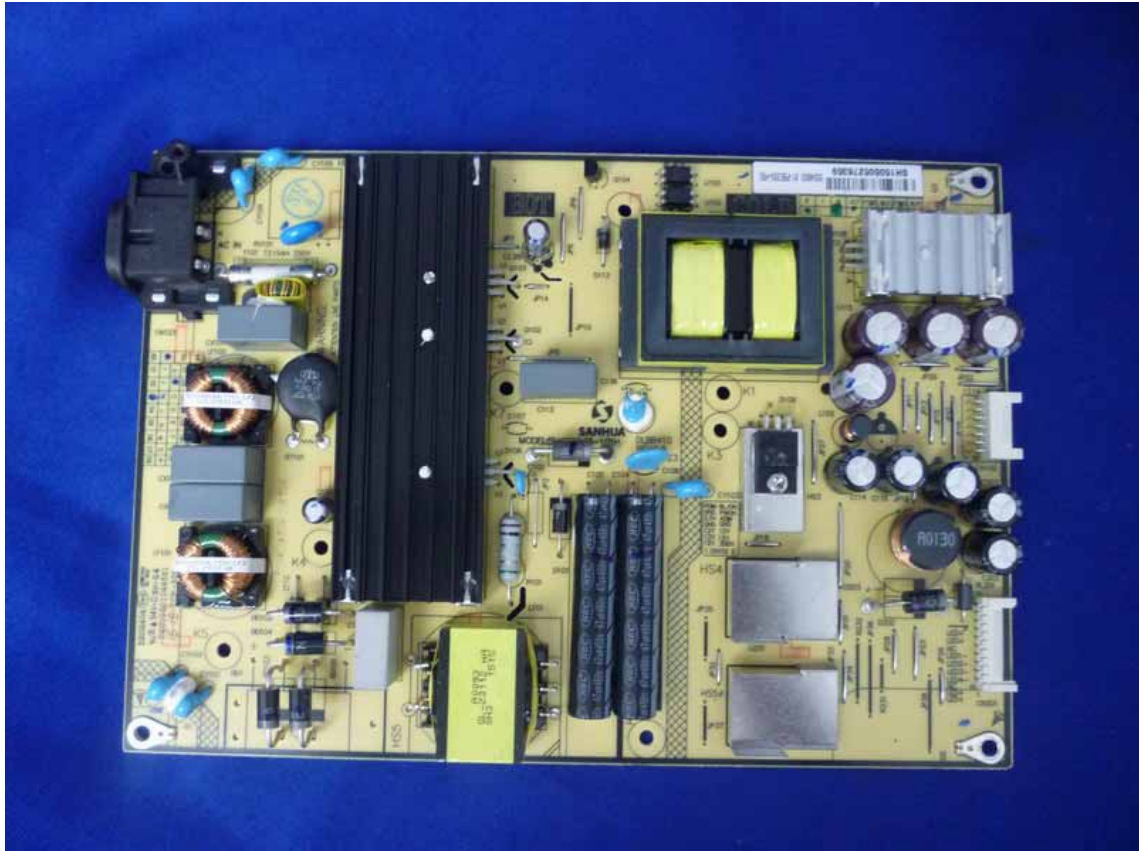
Figure 9 Frontside of the Power Board
