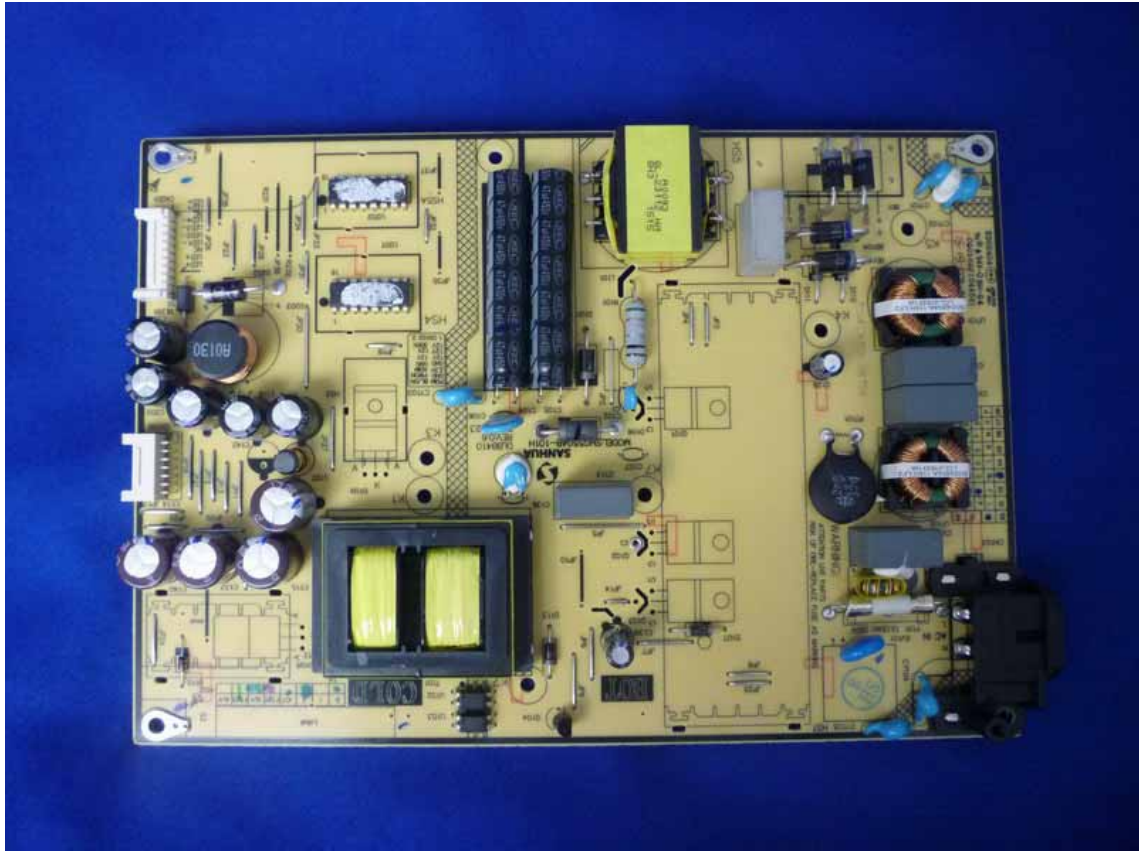
Figure 11 Frontside of the Power Board
