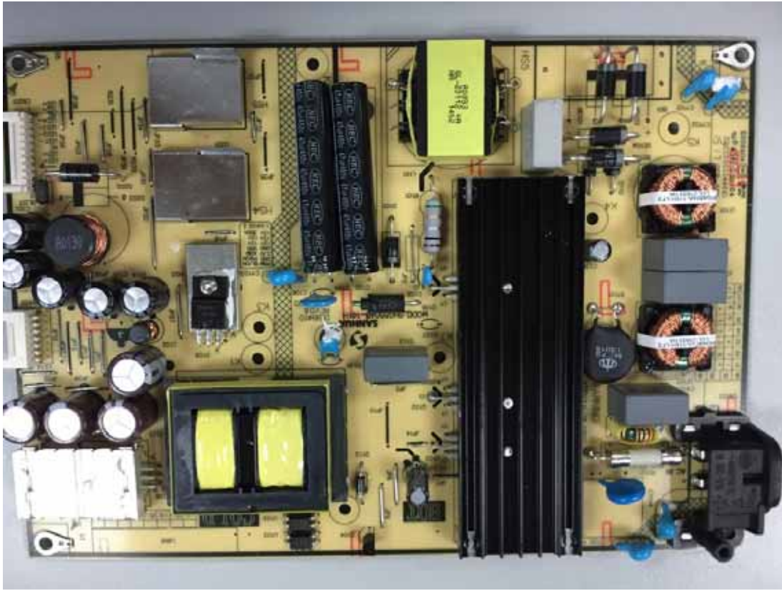
Figure 13 Frontside of the Power Board
