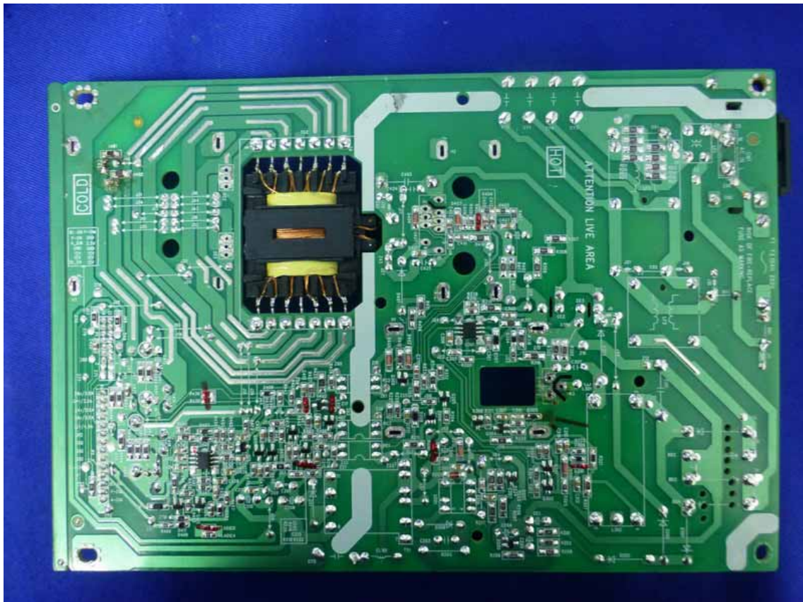
Figure 20 Backside of the Power Board
