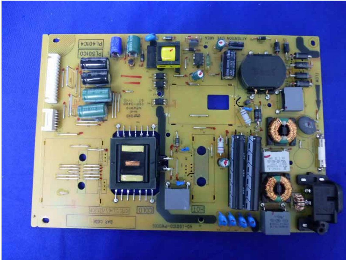
Figure 19 Frontside of the Power Board
