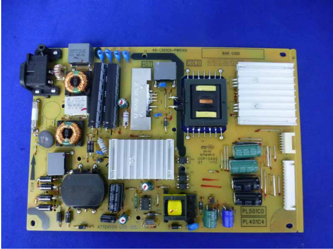
Figure 17 Frontside of the Power Board
