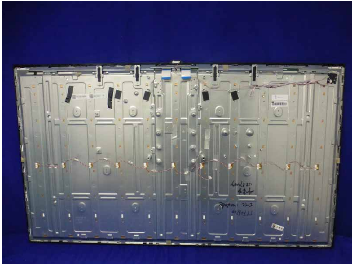
Figure 11 Backside of the LCD Panel
