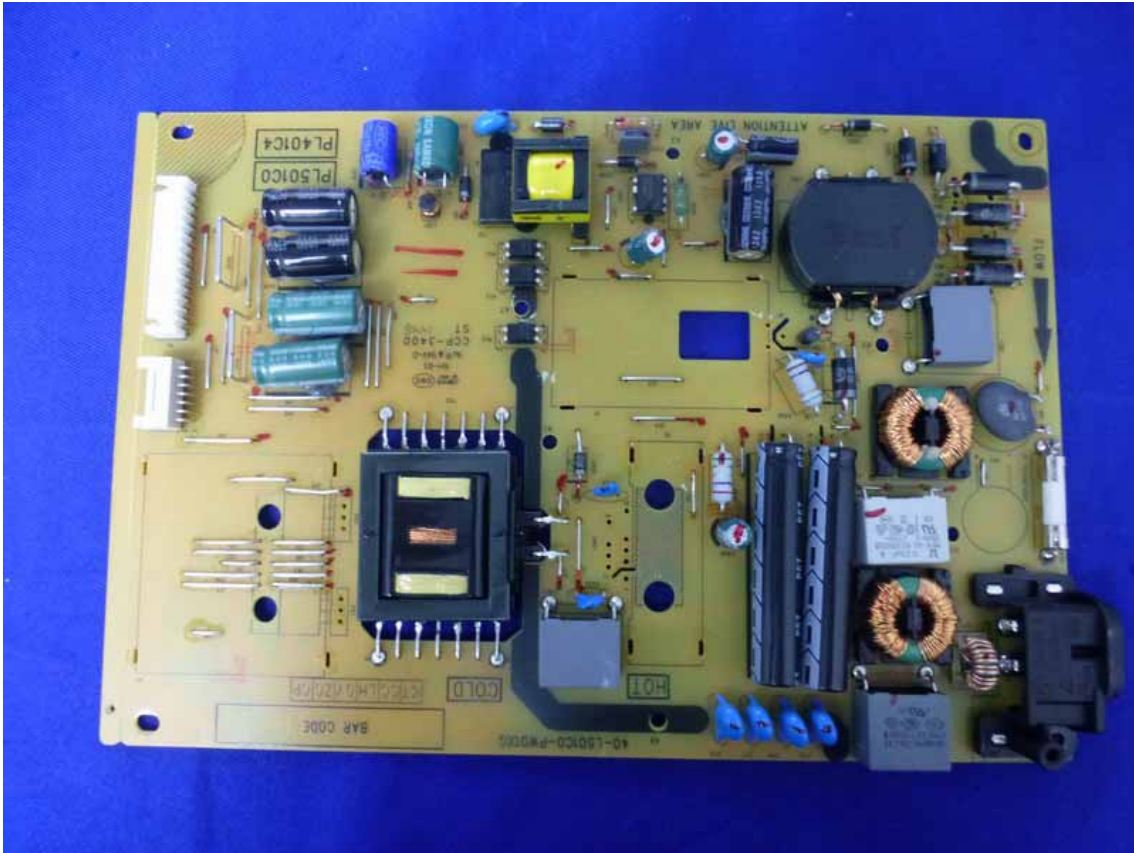
Figure 19 Frontside of the Power Board
