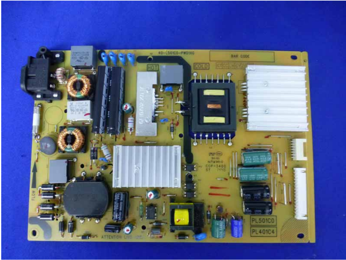
Figure 17 Frontside of the Power Board
