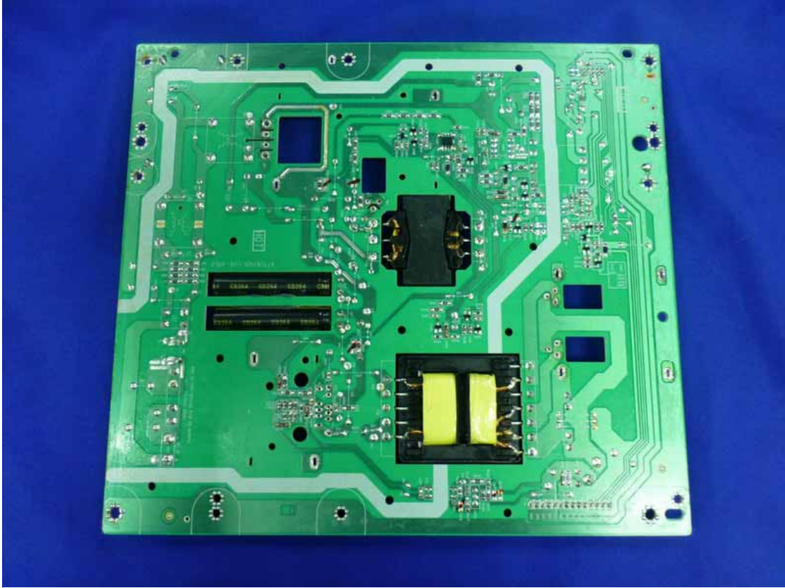
Figure 25 Frontside of the Power Board
