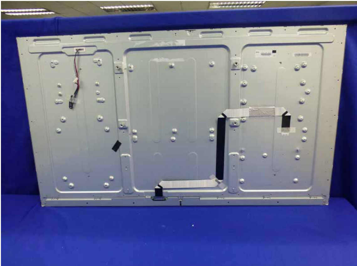
Figure 14 Backside of the LCD Panel
