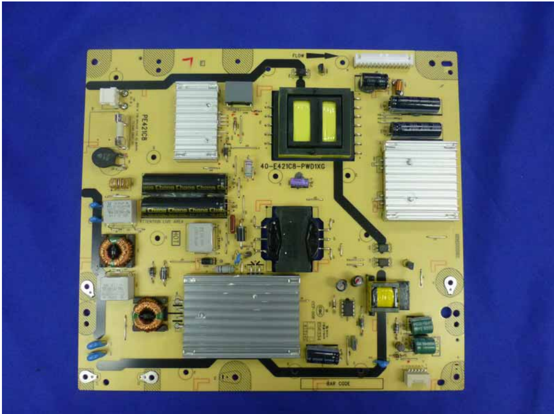
Figure 22 Frontside of the Power Board
