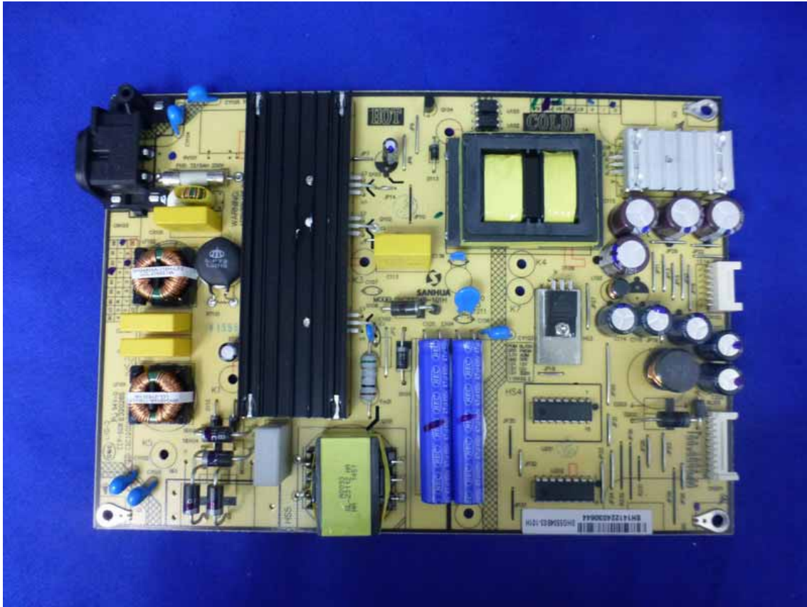
Figure 13 Frontside of the Power Board
