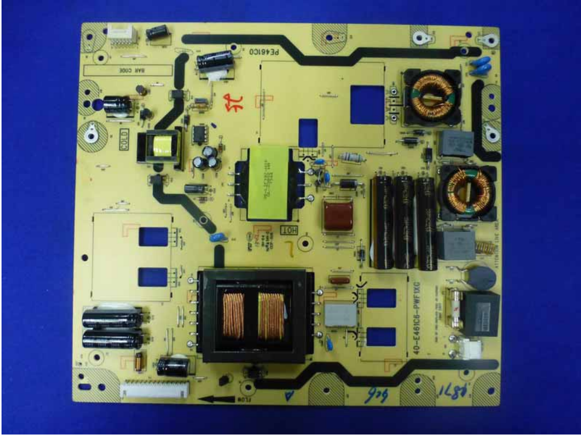
Figure 21 Frontside of the Power Board
