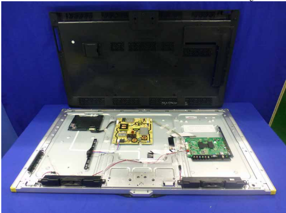
Figure 8 Inside Configuration of the EUT
