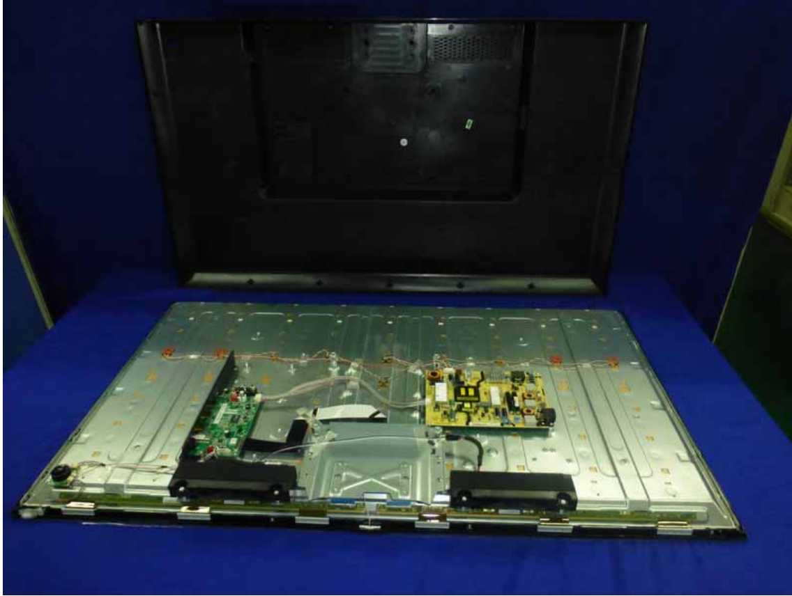
Figure 9 Inside Configuration of the EUT
