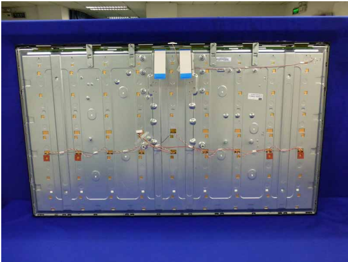
Figure 12 Backside of the LCD Panel
