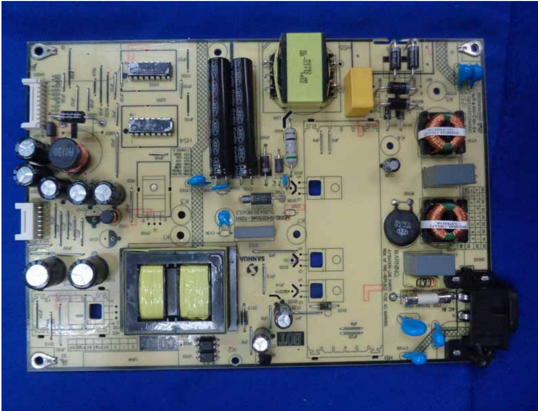
Figure 13 Frontside of the Power Board
