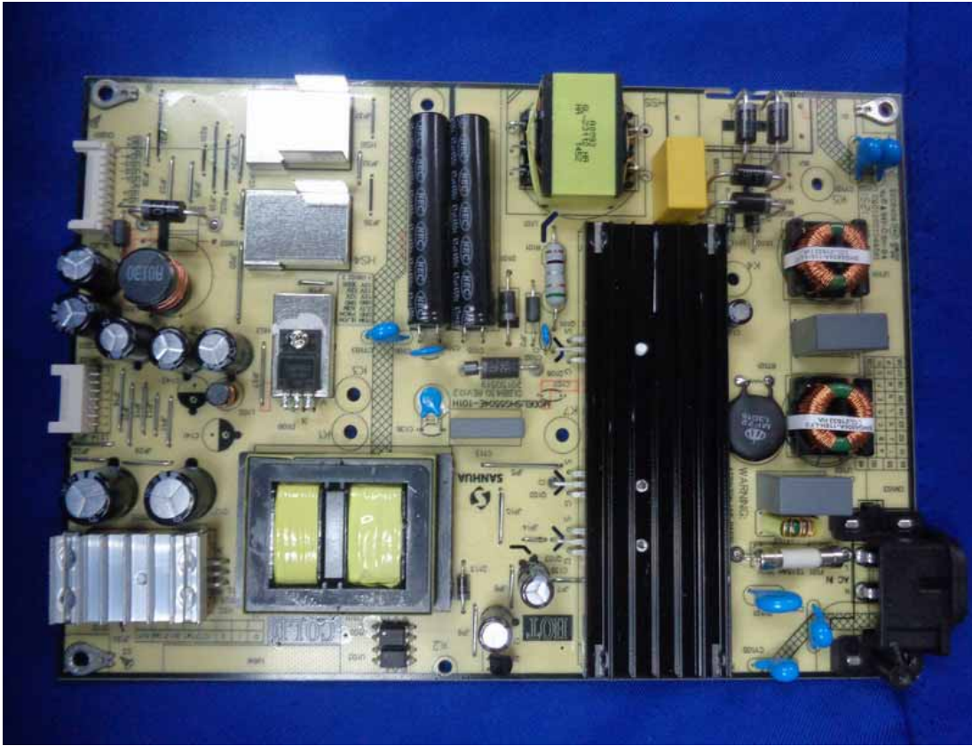
Figure 11 Frontside of the Power Board
