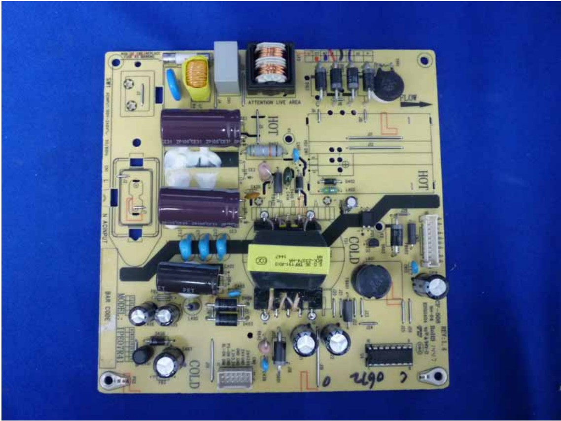
Figure 21 Frontside of the Power Board
