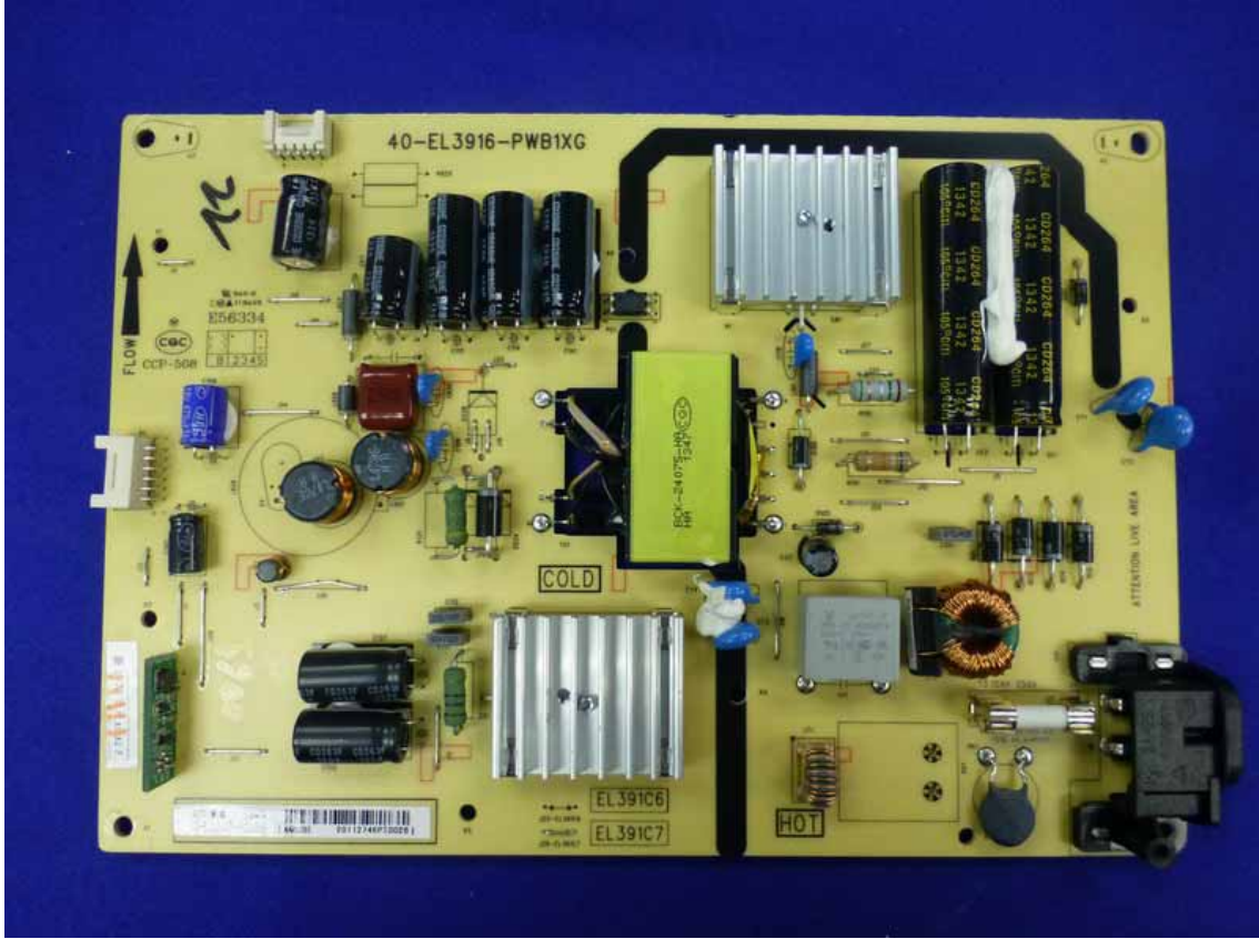
Figure 21 Frontside of the Power Board
