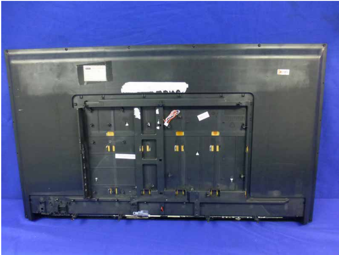
Figure 15 Backside of the LCD Panel
