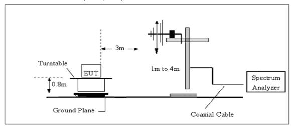
Radiated Emission Test-Up Frequency Above 1GHz
