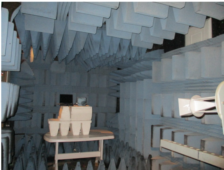
Radiated Emission Test, 18-26.5GHz
