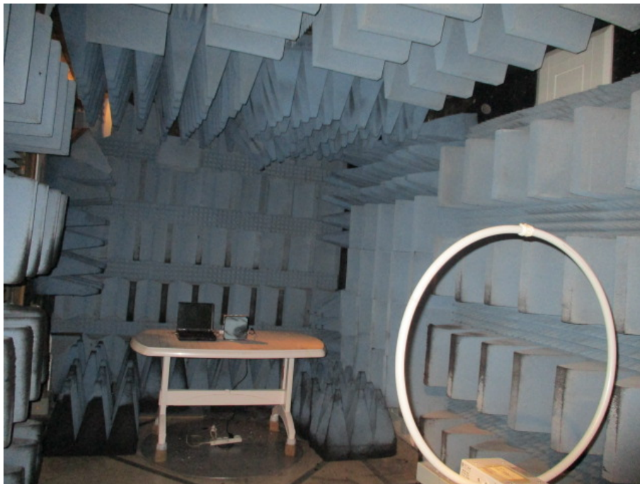
Figure 7. Radiated Emission Test, 0.009-30MHz
