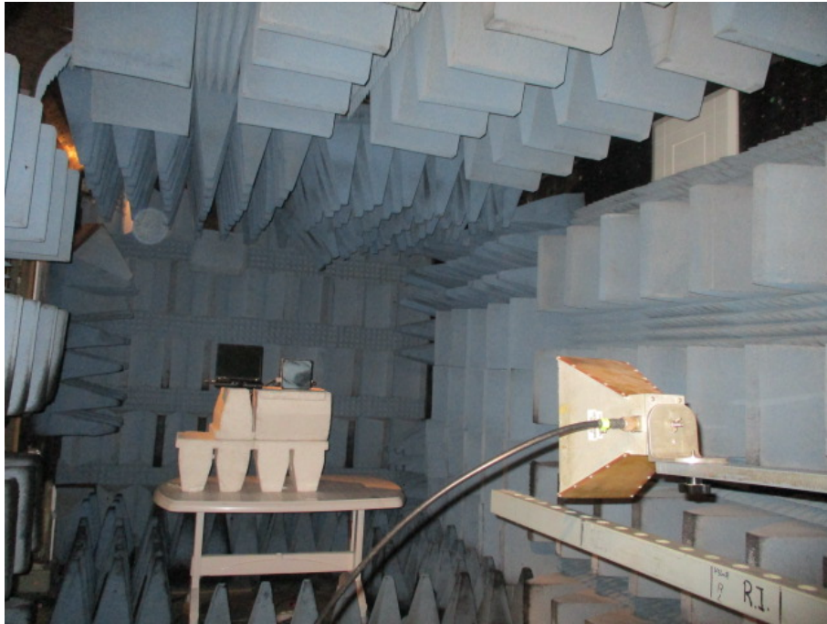
Figure 10. Radiated Emission Test, 1-18GHz
