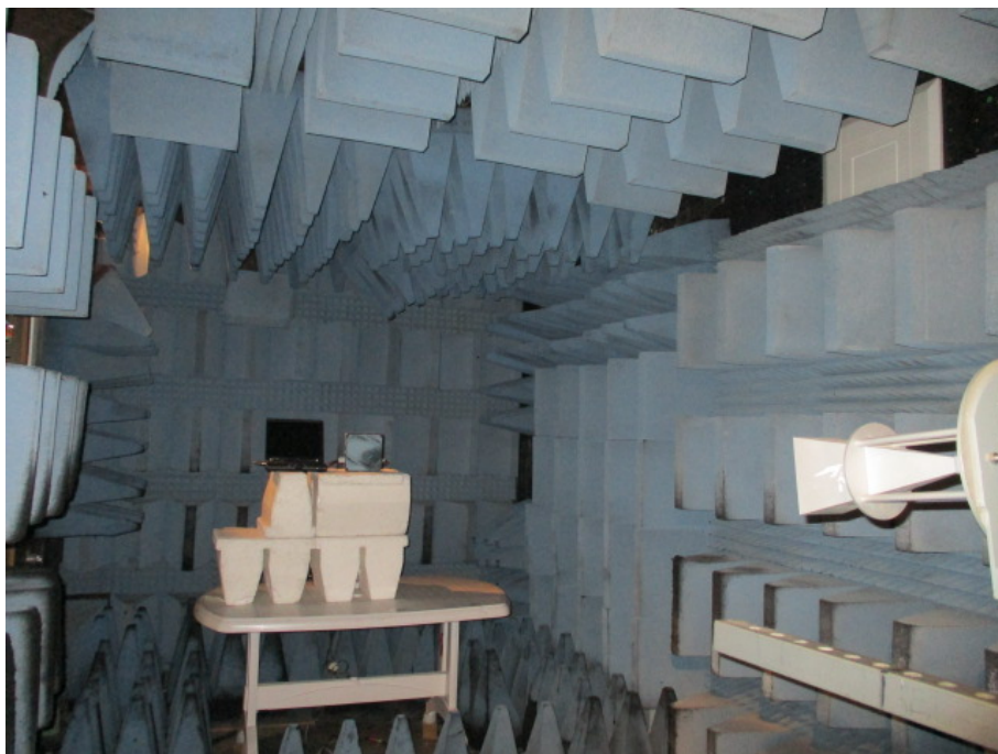
Figure 11. Radiated Emission Test, 18-26.5GHz
