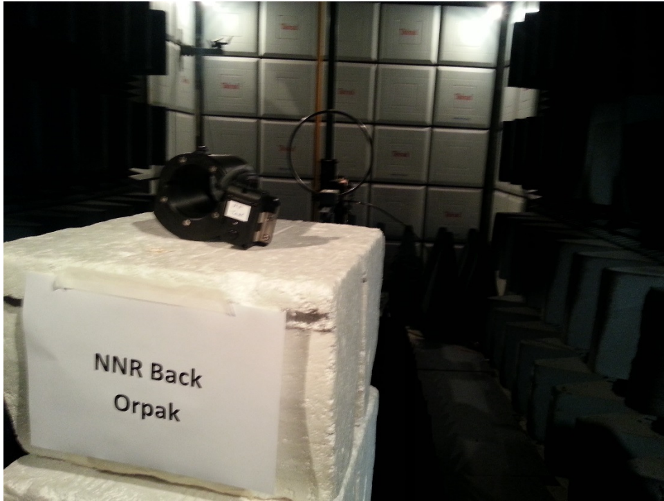
Figure 1. Fundamental and Radiated Emission Test Setup
