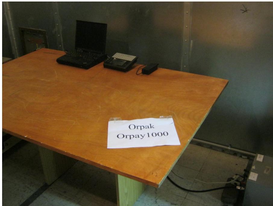
Figure 2. Conducted Emission from AC Mains Test Setup
