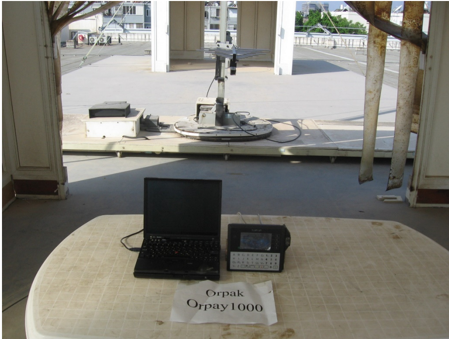
Figure 5. Radiated Emission Test
