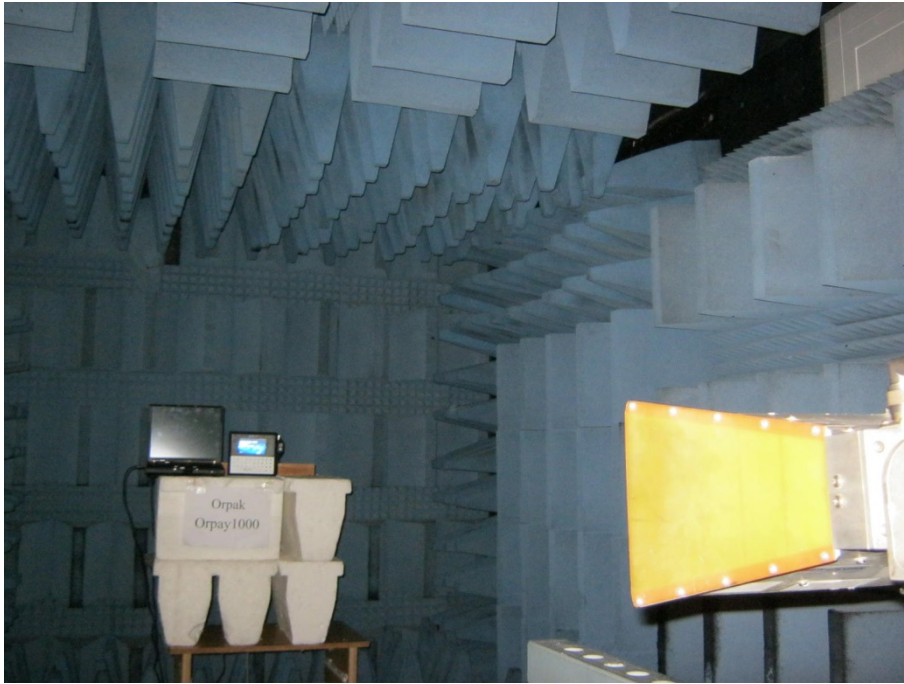
Figure 7. Radiated Emission Test
