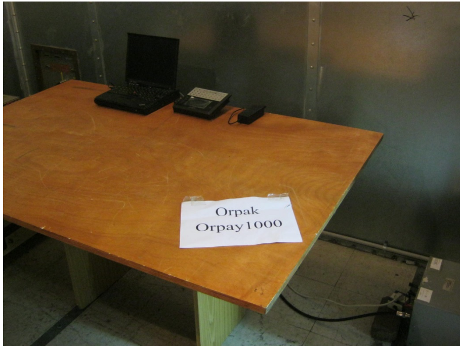
Figure 3. Conducted Emission Test
