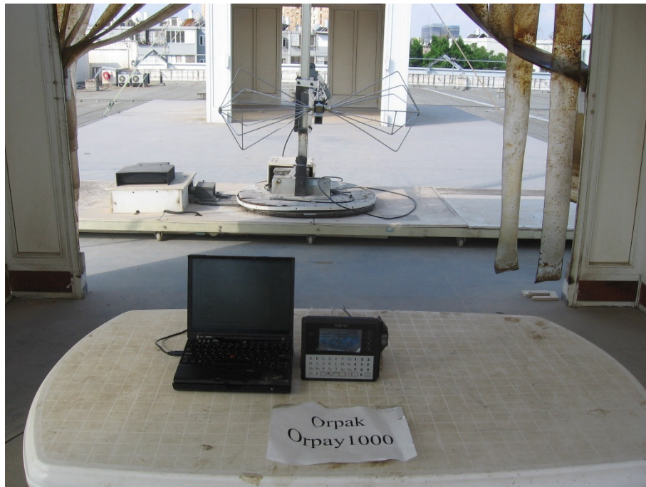
Figure 4. Radiated Emission Test
