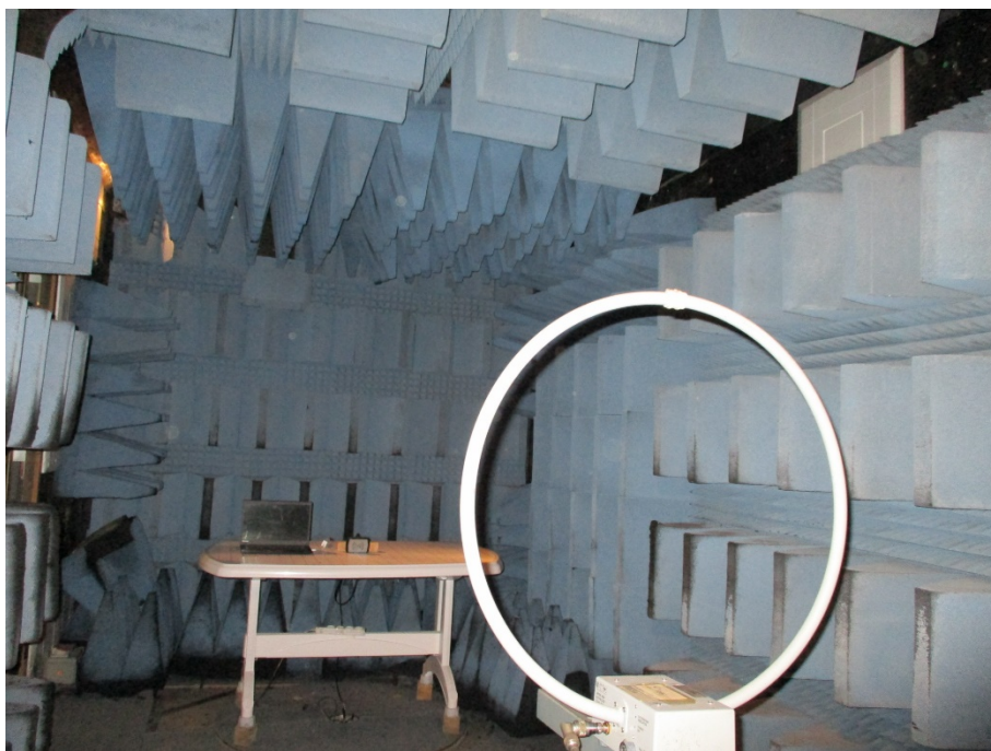
Field Strength of Fundamental & Radiated Emission Test Setup, 0.009-30MHz
