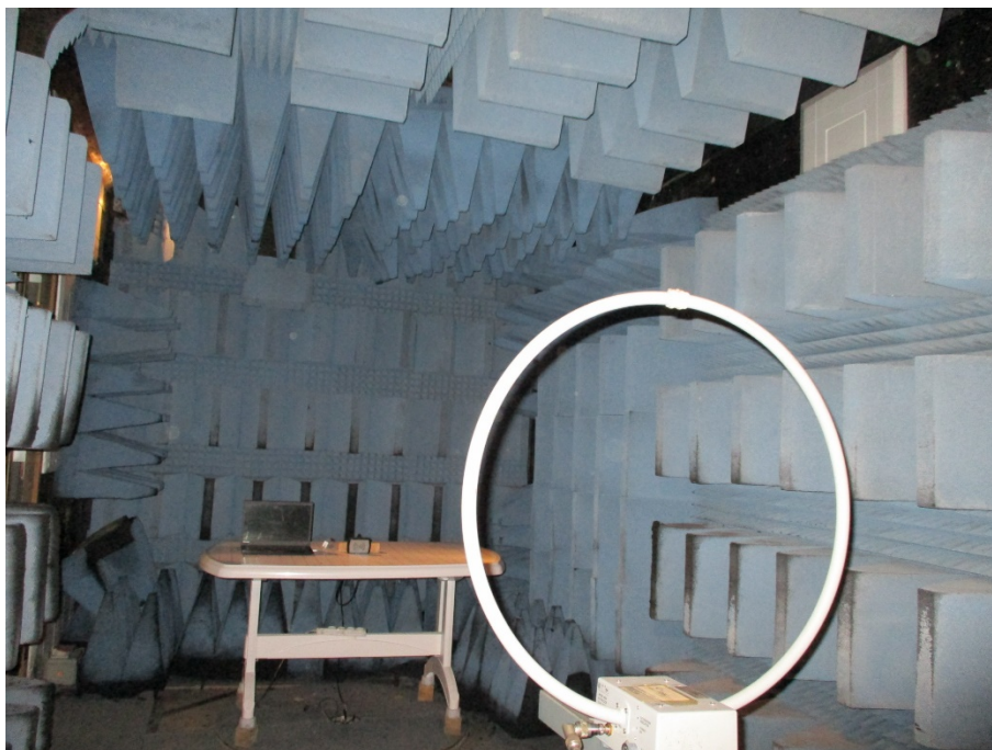
Figure 3. Radiated Emission Test Setup, 0.009-30MHz
