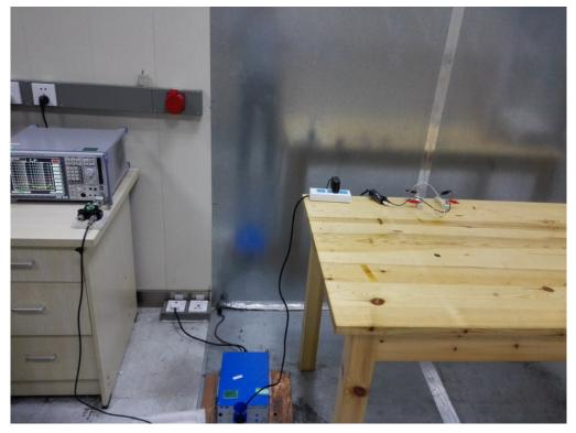
RADIATED EMISSION TEST SETUP BELOW 1G
