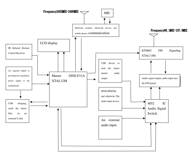
From the car cigarette lighter to provide power to the board after the regulated 5V power supply, and to the IPOD, IPHONE and other equipment charge, host-driven LCD display data,
