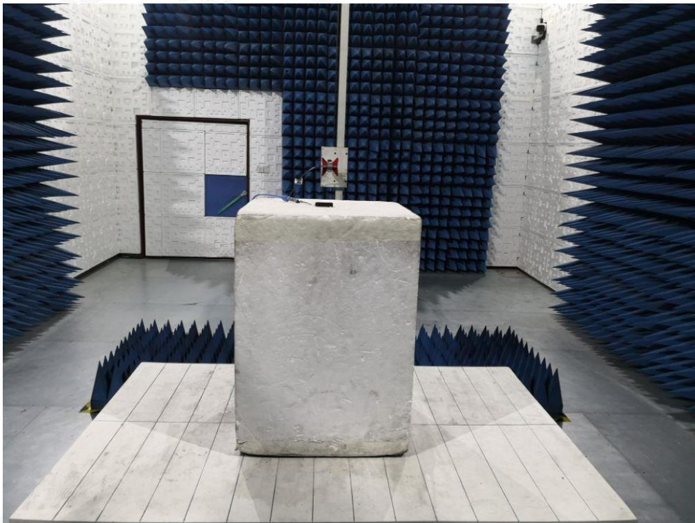
RADIATED EMISSION TEST SETUP ABOVE 1GHZ
