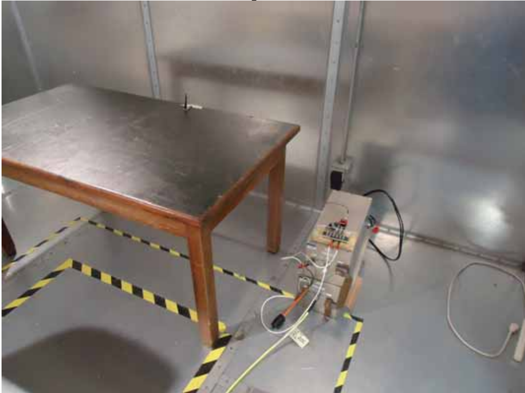
Test Setup for Conducted Emissions
