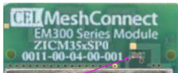
Capacitor C25 is placed vertically to use PCB trace antenna.
