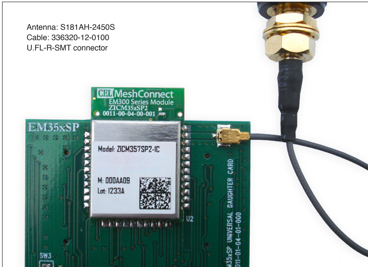
Figure 4. Implementation using connector, cable and external antenna
