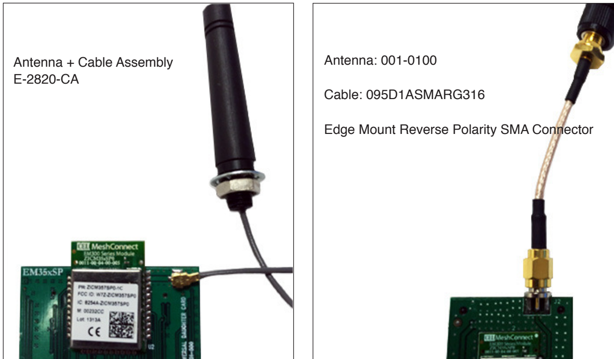
Figure 3. Implementation using connector, cable and external antenna
