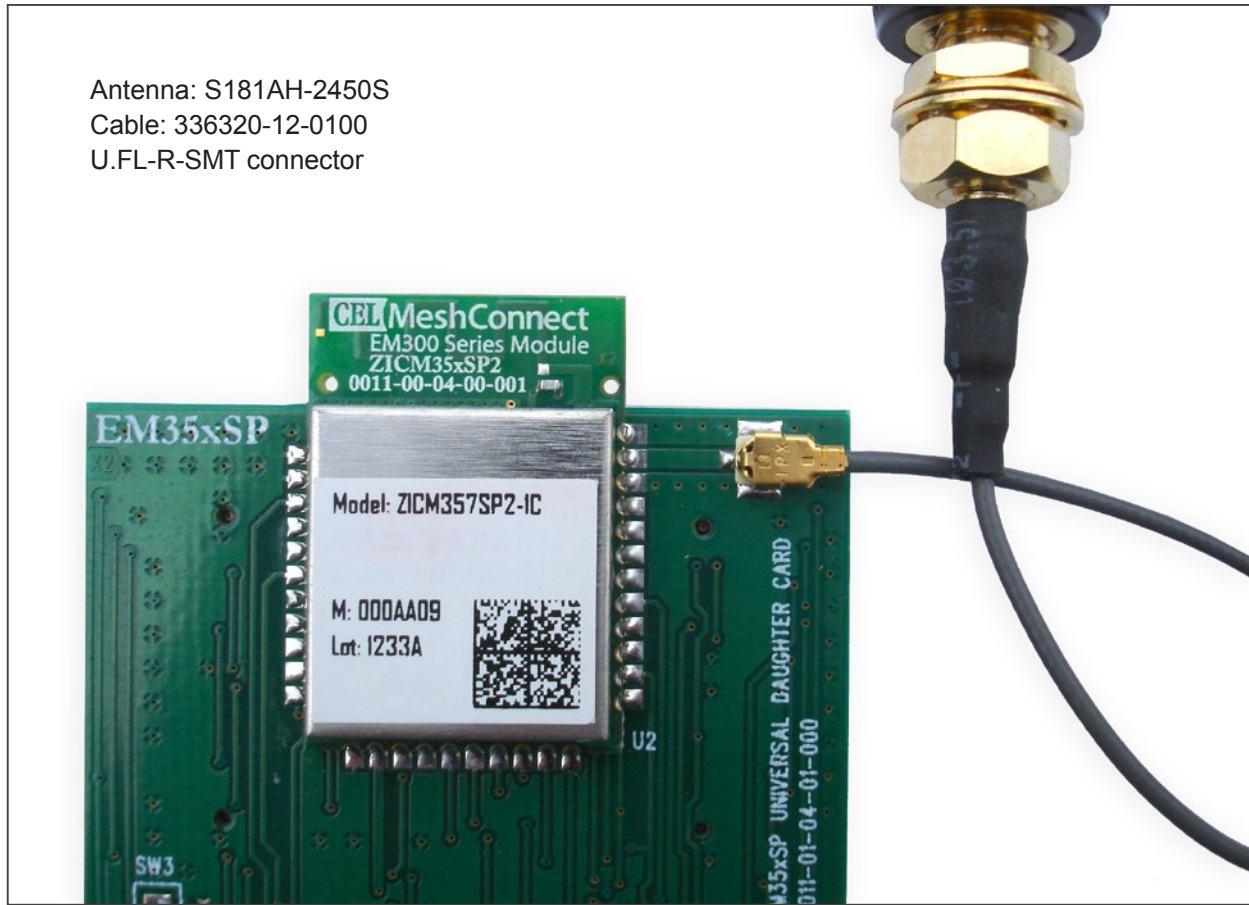
Figure 4. Implementation using connector, cable and external antenna
