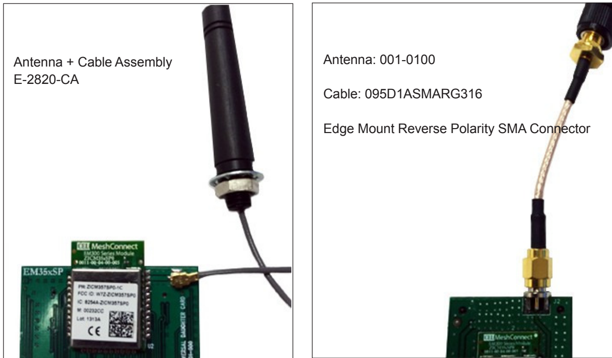
Figure 3. Implementation using connector, cable and external antenna
