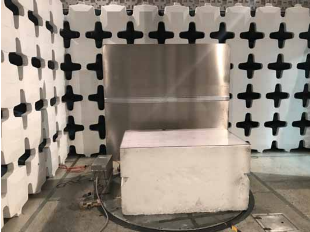
Photograph of the Conducted Emissions Setup
